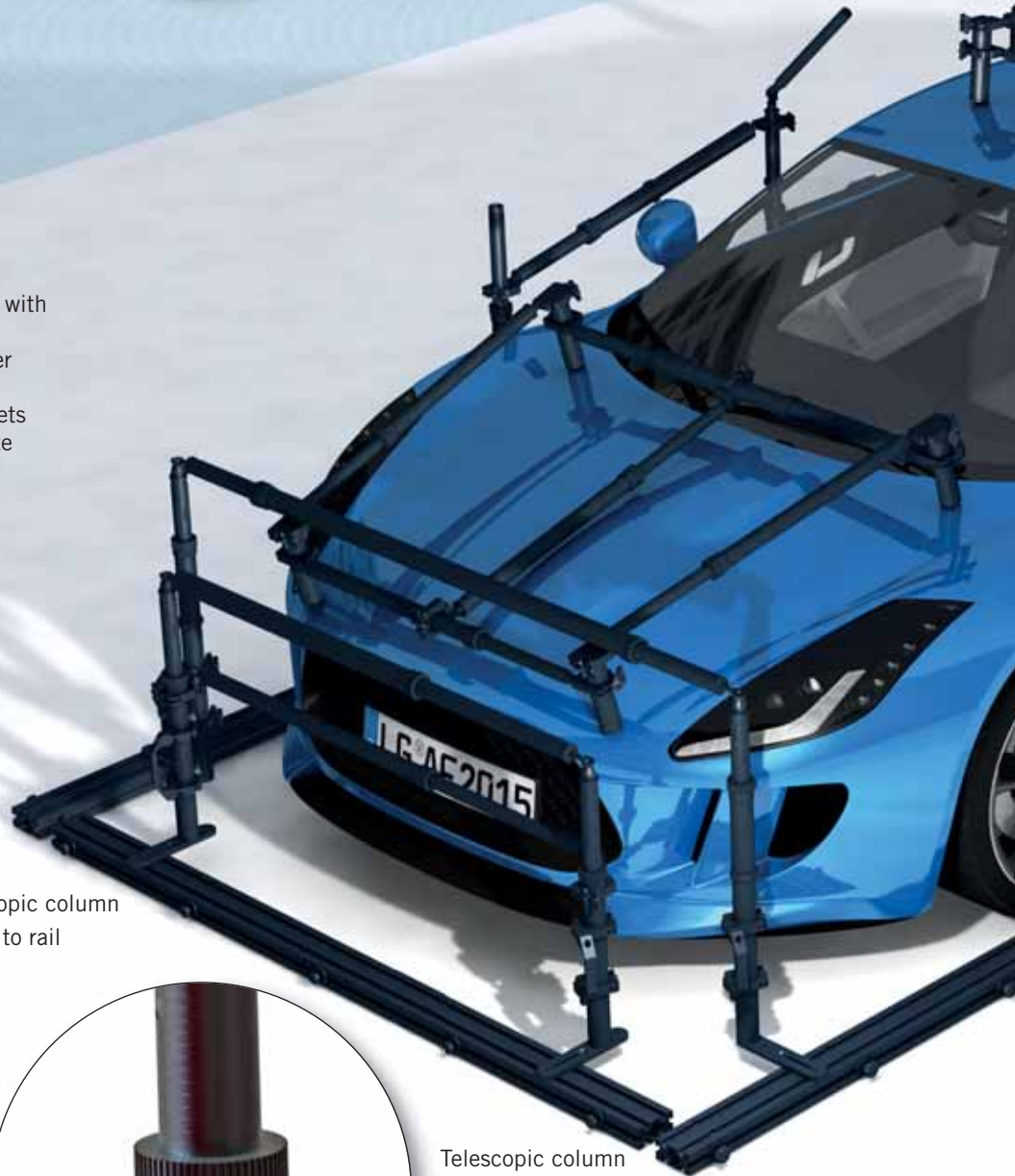
Cross struts in telescopic fashion with integrated targets
