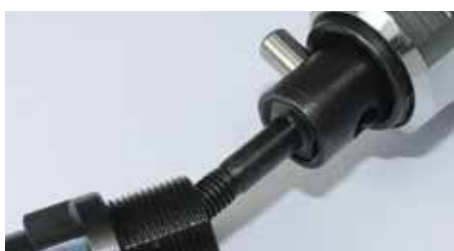
Quick-change system for the threaded mandrel.
